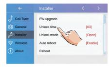
Step 3. The Installer Setup with keypad will show up. Then input number from 01-99 and touch OK to set the unlock time as 1-99 seconds.
