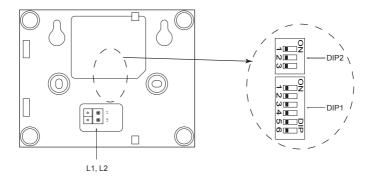
L1,L2:Bus terminal. DIP1(Bit1~6):Used to User Code setting. DIP2(Bit1~3):Used to Slave Monitor Address or Extended Address setting.
