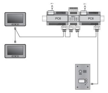
3.2 Router Mode: In this mode, the system can connect up to 8 BDUs, and each BDU can connect up to 32 monitors.
