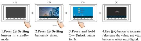
\*Note: Press and hold 😳 Setting button for 3s on panel in standby mode to enter the installation setting page in shortcut.
