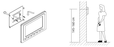
Use the screws to fix the Mounting Bracket on the mounting box.(fitting accesories includes a Bracket (Two pieces of 4X25 screws are needed for fastening the Mounting Bracket), Special 2 wire connectors to connect with Monitor)
